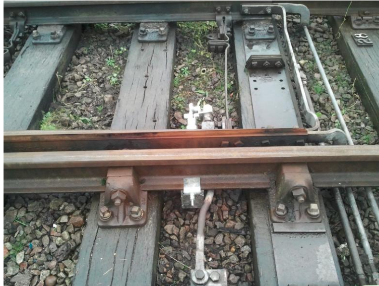
Figure 4.6: Autochock Installation
