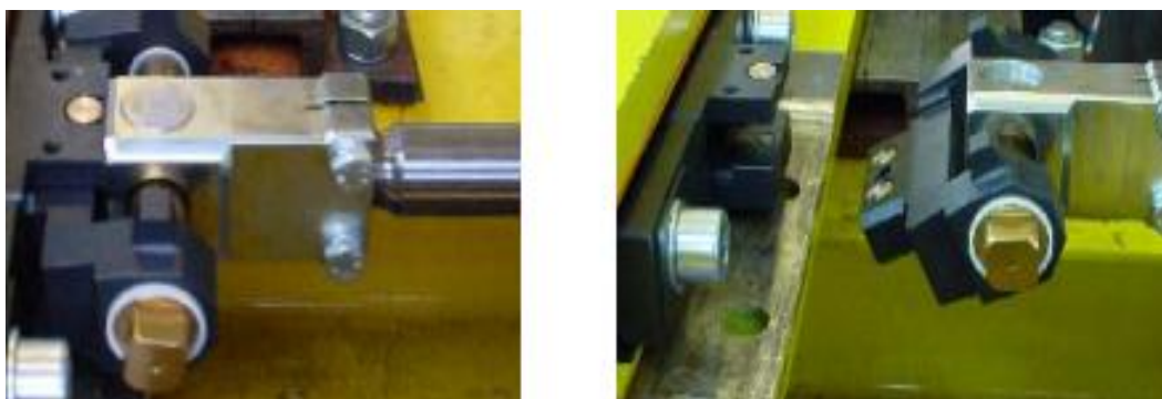
Figure 3.3: Operation of the Break-Out-Device (BoD)
