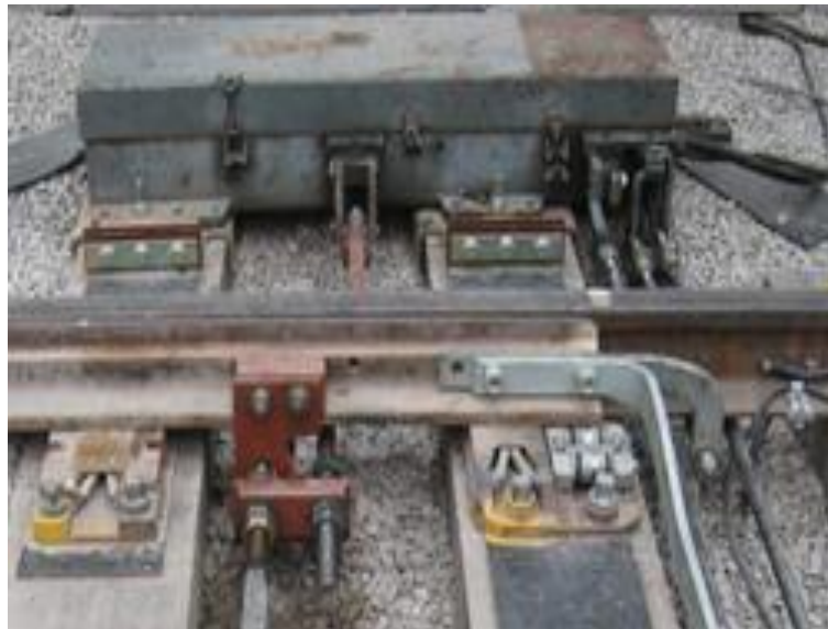
Figure 3.9: Style 63 Points Machine photograph
