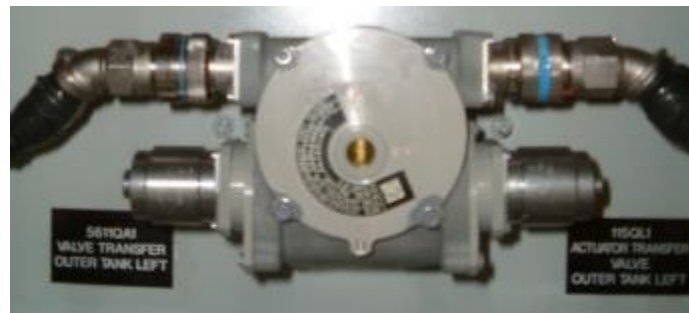
Figure 9.8: Fuel valve twin-motor actuator
