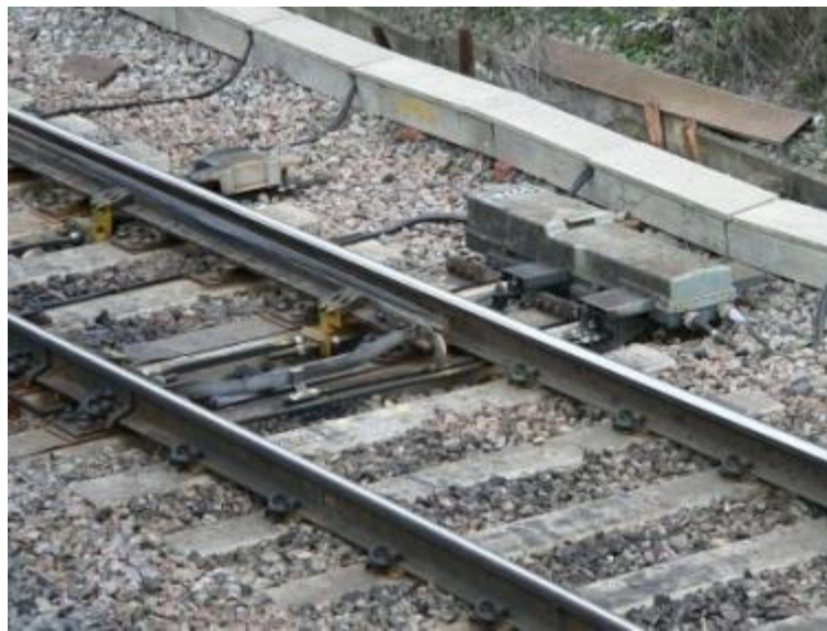
Figure 3.6: HW Points Machine photograph
