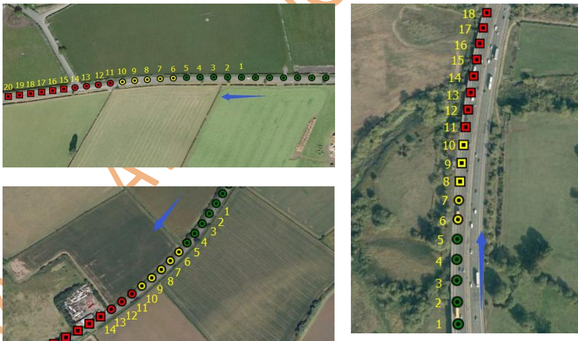
Figure: 37. Fixes switch to unfixed solutions when the time latency increases (numbers closed to each epoch symbol are differential latency in second)
