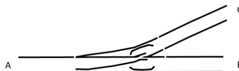
Figure 13.1: Sketch of a switch and crossing including breathing sections
