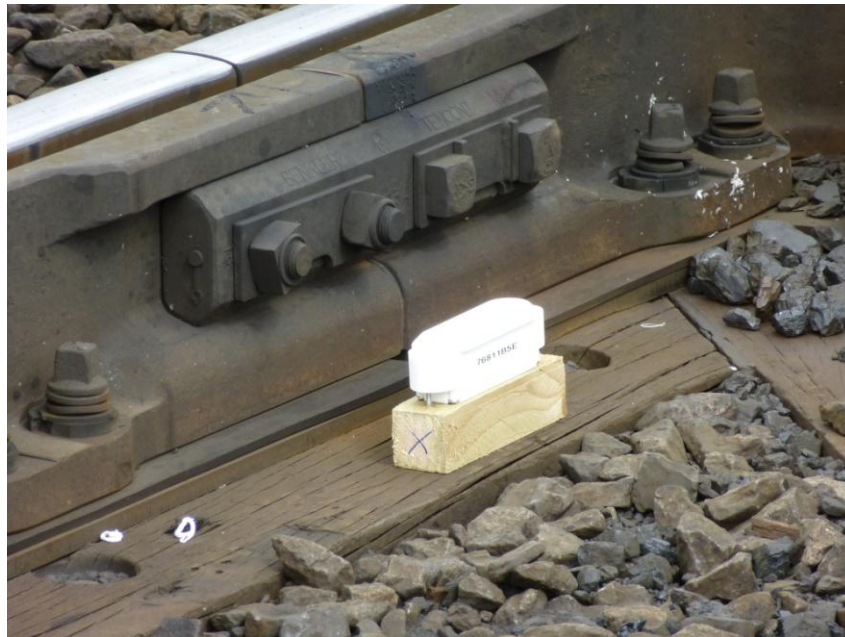
Figure 11.2: Wireless sensor fixed to existing timber sleeper for demonstration purposes
