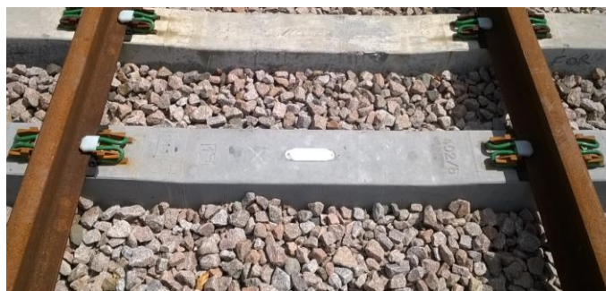
Figure 11.1: Wireless sensor embedded in a purpose-built concrete sleeper
