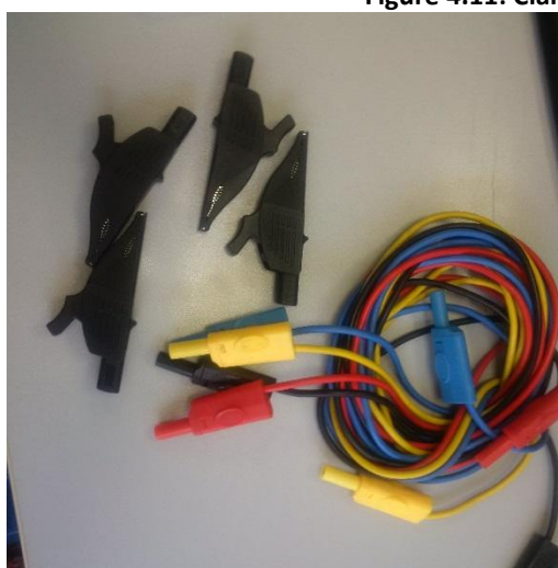
Figure 4.12: Voltage measurement sensors and conductors
